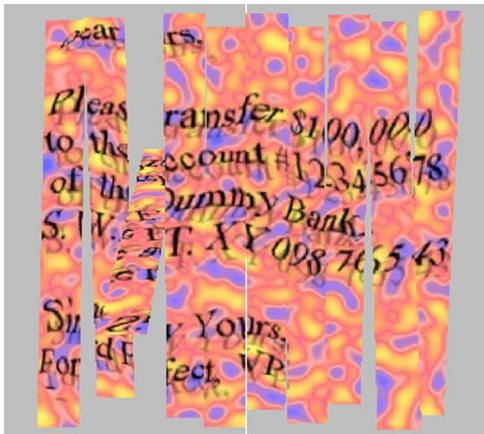
Fig. 2. A snapshot of the “Flying Pieces” animated captcha. The distorted text is projected onto a color patched surface which is cut into stripes. The stripes rotate in 3D and at the instant are close to coming together, so that the document can be recognized
