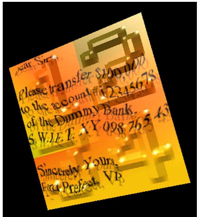
Fig. 2. A snapshot of an animated CAPTCHA for document authentication. The distorted text is projected onto a morphing surface. At the instant, the code “1234” can be recognized on the surface.
